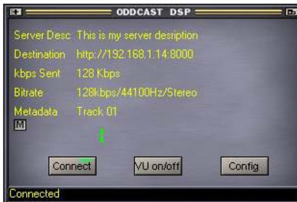
Now your streaming has begun! You can control what bitrate you are streaming at – view metadata (information’s on the streamed file) and finally a VU-meter (showing left-right audio channel volume. You may switch the meter off)
